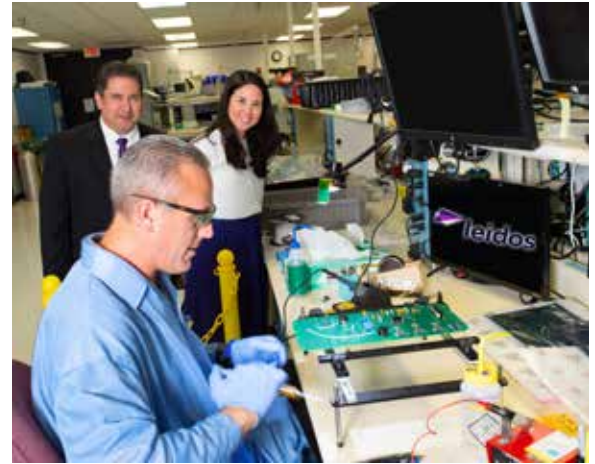
Inside the Leidos' Engineering Lab, Ernest Sanchez and Tanya Hanway observe as Lee Risinger solders components onto the circuit board for a power supply to prepare for use in the ISS.
